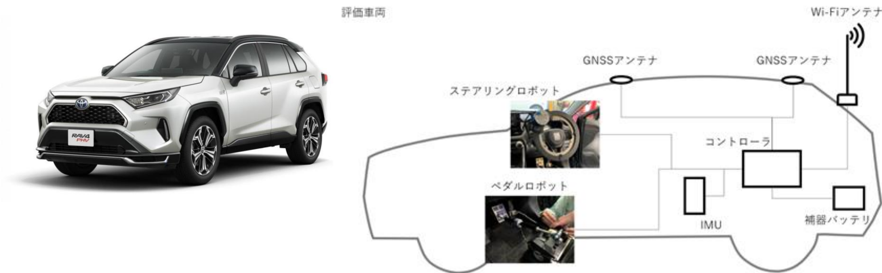
Fig.5 Evaluation vehicle equipped with a steering and pedal robot
