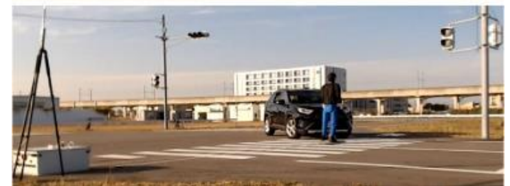
Fig.10 AEB evaluation of a collision scene with a pedestrian crossing when turning left at an intersection
