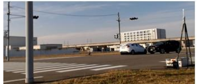
Fig.8 AEB evaluation of a collision scene with a vehicle going straight ahead when turning right at an intersection
