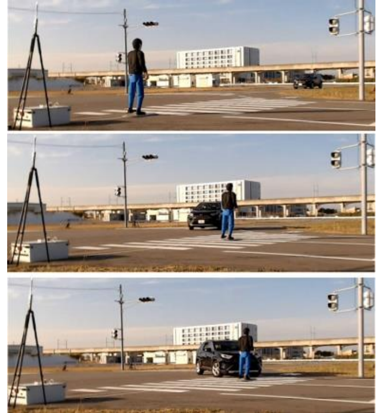
Fig.11 Pedestrian D. and Vehicle trajectories of AEB evaluation of a collision scene with a pedestrian crossing when turning left at an intersection
