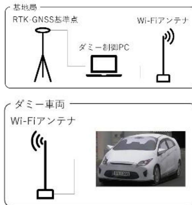
Fig.4 Control methodology of a dummy car running plate
