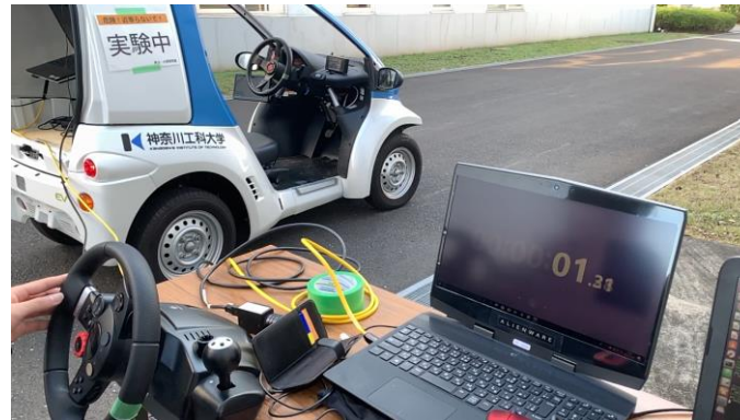
Fig.5 Delay time measurement of steering wheel angle
