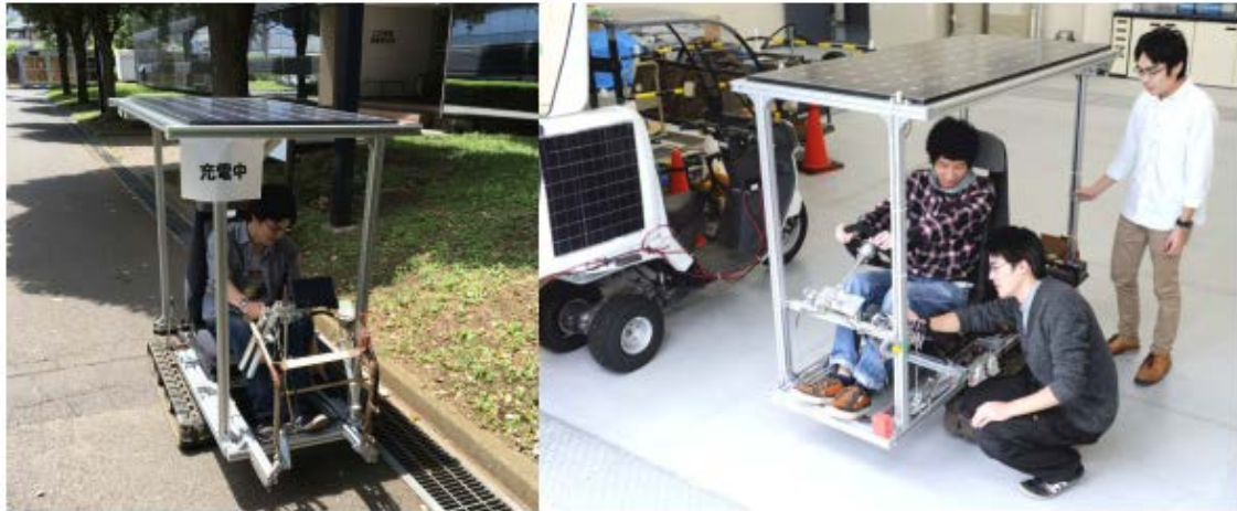
Fig. 4: Converted crawler-type solar EV (Left: outdoor charging in summer, Right: in a garage in winter)
