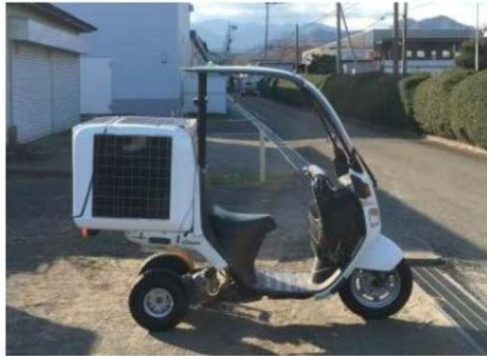
Fig. 1: Solar EV (EV conversion of HONDA GYRO CANOPY)
