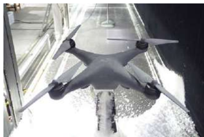
図 4.1.1.1.2. URAV with coated surface placed in wind tunnel
