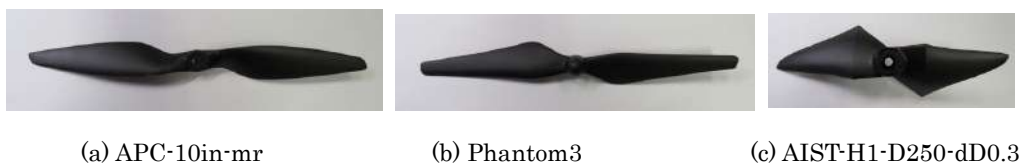
図 4.1.1.1.1. Rotor blade used for snowing test
